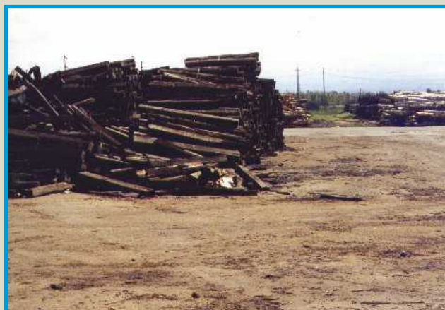
Railroad ties and logs for fuel at Wheelabrator Shasta Energy Company, Anderson, California. The power plant is allowed to burn not more than 25 percent railroad ties; burning plywood, particleboard, or plastic laminates is not permitted.
