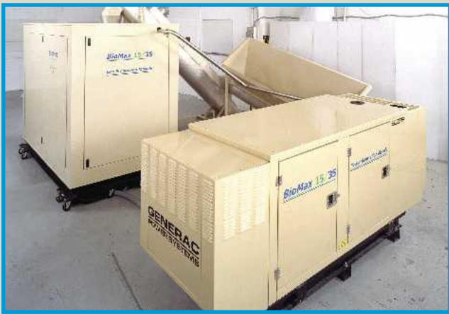
The BioMax 15 is a prototype combined heat and power system developed by Community Power Corporation, Littleton, Colorado. This is a state-of-the-art, transportable, fully automated, and environmentally friendly system. It can provide heat and power to small businesses, rural homes, and greenhouses.
